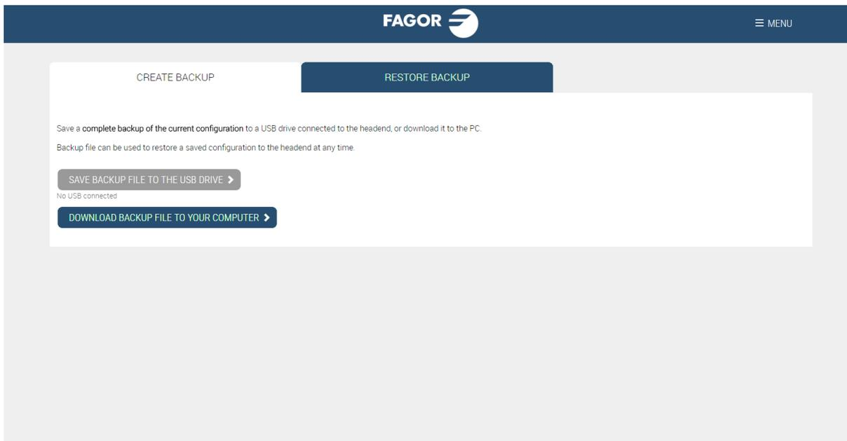
Select CREATE BACKUP tab to download a file with the complete configuration of the headend. The file can be downloaded on a USB drive or on the computer itself.
