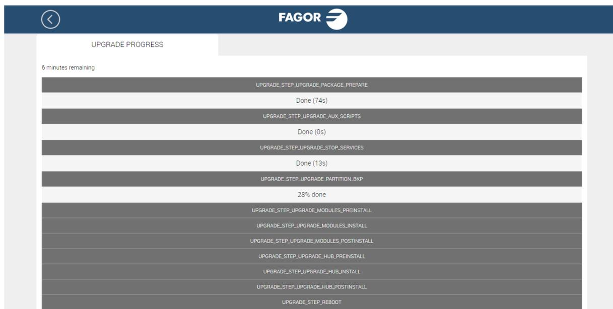
This screen shows all the steps of the upgrade, indicating which have already been made, how long have needed and the percentage of progress of the current step.
