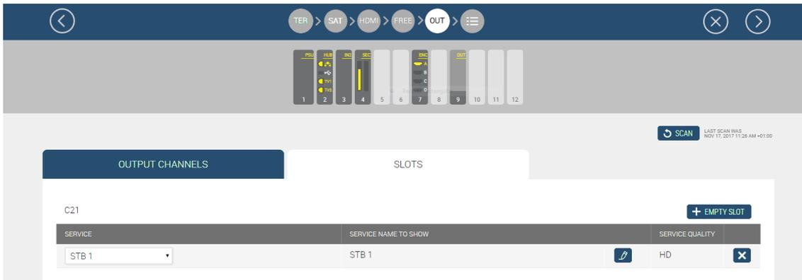
This tab allows to assign which content is conveyed by each slot and what name will be displayed by the TV. For more information, see Ikusi Flow Slots Configuration Guide.
