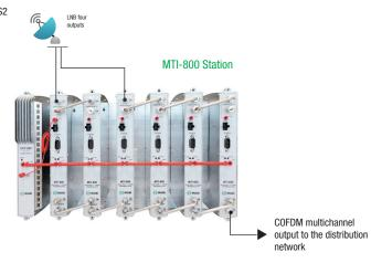
A satellite dish aimed at a satellite and connected to equipment composed of 6 transmodulators MTI-800 and a CFP-700 source, allows us to tune in to a large number of open channels, both regional and international.
