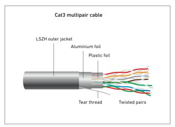
STEP 2. Remove the coverings from the multipair telephone hose until the twisted pairs are exposed.
