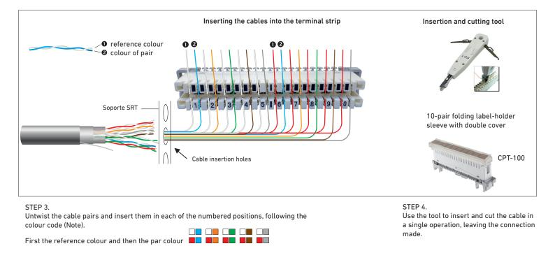
(Note) The pairs of wires should remain twisted for as long as possible and should be untwisted to the correct length. This is because twisting is precisely what prevents interference or keeps it to a minimum.
